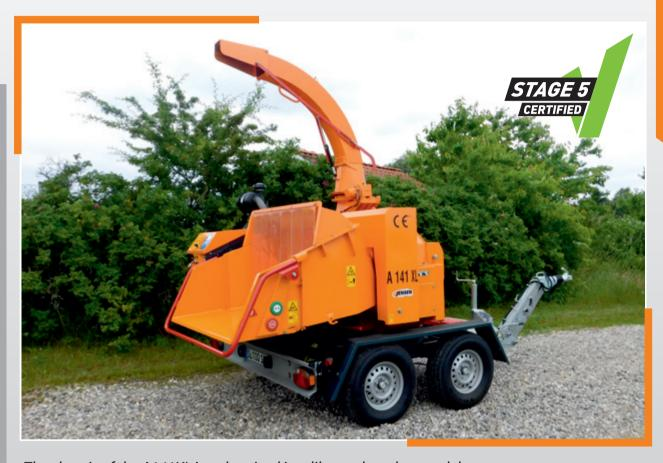
The chassis of the A141XL is galvanized just like on the other models. Despite the size of this machine, regular maintenance work can be carried out quickly and easily.
