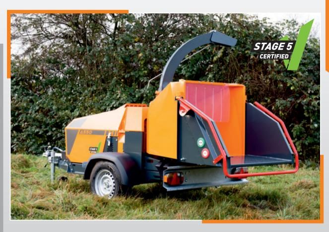
This new model has a reliable Yanmar engine with DPF and common rail technology. The accessibility of the engine is excellent due to the newly developed hood.
